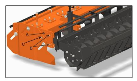
Operator can adjust the roller height in eight different positions, by inserting the two adjusting pins (B) into the holes immediately above and below the roller's swinging arms, according to the desired working height.
