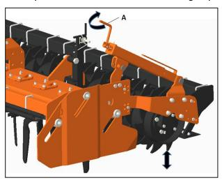
The position of the roller frame relating to the swinging arms affects the adjustment of the working depth.
