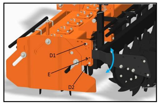
This configuration can be useful in case the machine meet an obstacle during operation, allowing the machine to overcome it without damaging the roller, thanks to the swinging arms, and obtaining a nearly uniform leveling of the ground.
