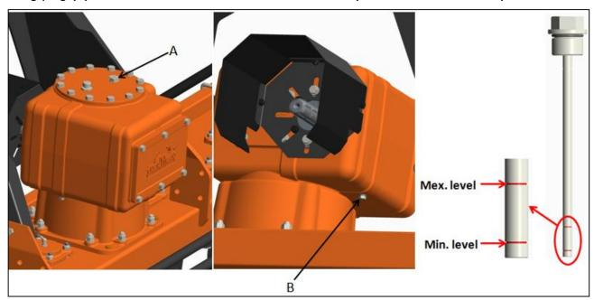
If the mark is below the minimum, fill up oil till the correct level is restored.
