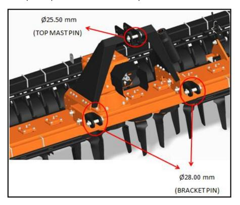
If the dimension of the pins is not corresponding to Category 2, contact the Manufacturer or the Dealer to obtain the pins of right dimension.
