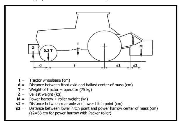
If the machine is combined with other machines (fertilizers spreaders or seeders), the ballast check must be done considering:
