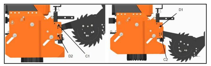
The roller can be left in floating configuration, free to follow the ground contour, by positioning the adjusting pin (D2) in a hole lower to position (E) immediately below to the connecting arm, or by removing it altogether.
