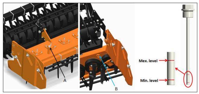
If the mark is below the minimum, fill up oil till the correct level is restored.
