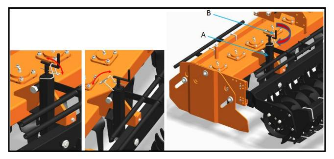
It is recommended to set the bar position at 4-5 cm higher compared to the position of the roller on the ground.
